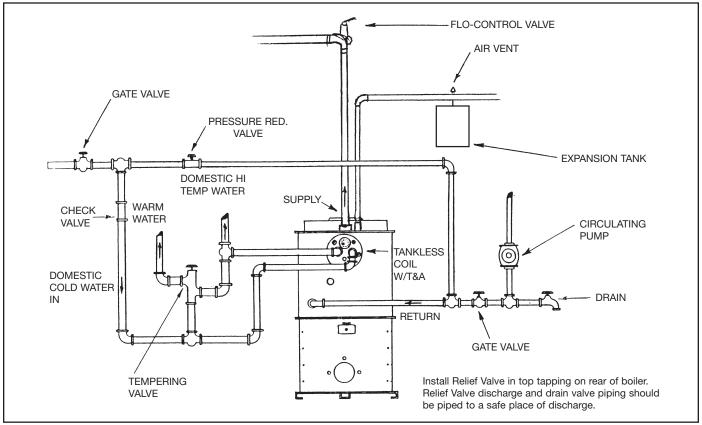
Figure 3. Boiler Piping
